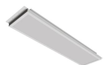
The Tegra LED panel is a bespoke modular luminaire designed to fit SAS330 ceilings. The body is made from powder coated steel giving a screwless appearance from under the ceiling. The diffuser is made from high efficiency PMMA which gives the luminaire optimum performance.
