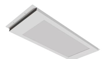
The Tegra LED panel is a bespoke modular luminaire designed to fit SAS330 ceilings. The body is made from powder coated steel giving a screwless appearance from under the ceiling. The diffuser is made from high efficiency PMMA which gives the luminaire optimum performance.
